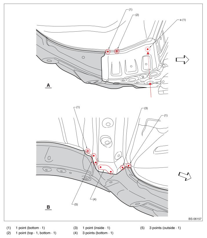
Note: Remove part "a" with a long spot cutter inserted through the hole indicated by the red arrow.
